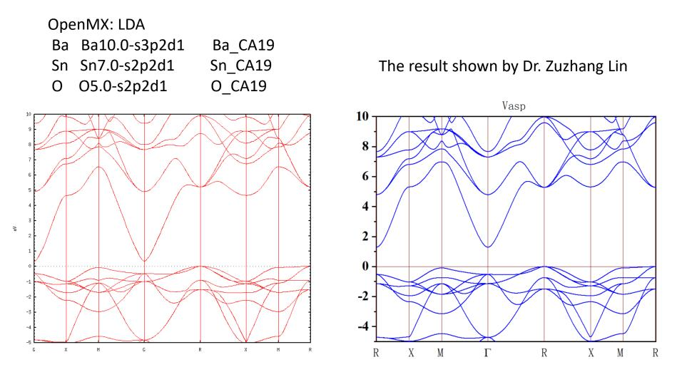
The overall feature of the band structure of BaSnO3 calculated by both the codes looks similar. The band gap by OpenMX is ~ 0.4 eV, which seems to be smaller than that by VASP. However, the band structure by calculated by VASP, shown at <u>https://materialsproject.org/materials/mp-3163/</u> also exhibits the band gap of 0.395 eV.
